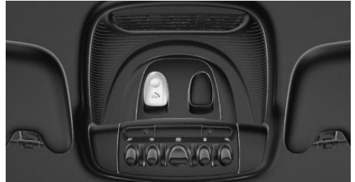
SOS button in the roofliner
