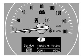
The remaining driving distance and the date of the next scheduled service are briefly displayed in the speedometer immediately after you start the engine or switch on the ignition.
