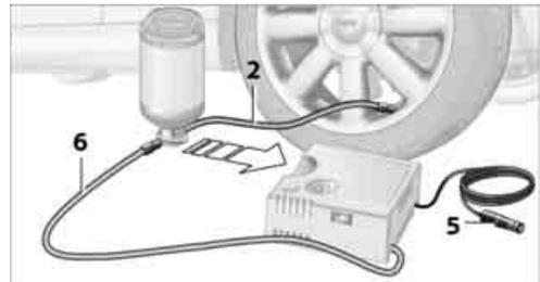
4. Unscrew the dust cap from the valve of the defective wheel and screw the filling hose 2 of the sealant bottle onto the valve.
