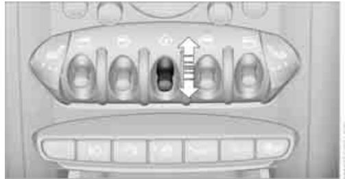
The switch locks or unlocks the doors and lift-gate when the doors are closed, but the anti-theft system is not activated. The fuel filler flap remains unlocked\*.
