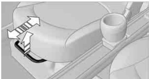
1. Pull the lever and slide the seat into the desired position.
