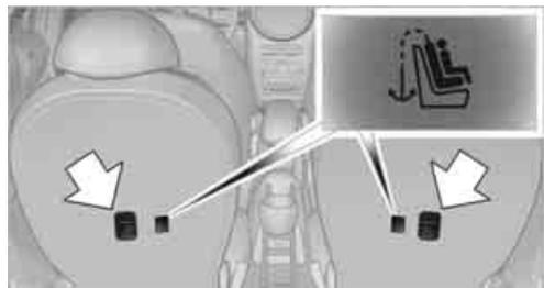
There are two additional anchors for child restraint systems with tether straps, arrows.
