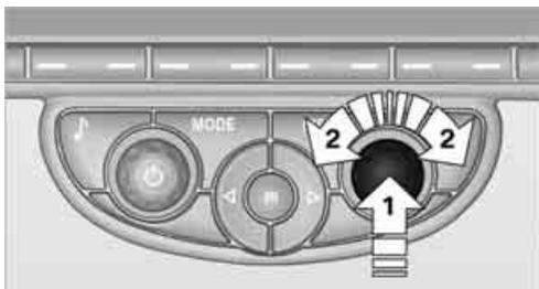
2. Press the knob, arrow **1**, to confirm a highlighted function.
