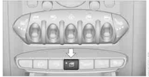
With the safety switch, you can prevent the rear windows from being opened or closed via the switches in the rear passenger area, by children, for example.
