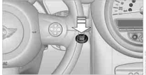
Press the Start/Stop button to switch radio readiness or the ignition on and off. Do not depress the brake or clutch while doing so.
