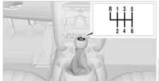
**!** When shifting into 5th or 6th gear, press the gearshift lever to the right. Otherwise, the engine could be damaged if you inadvertently shift into 3rd or 4th gear. ◀
