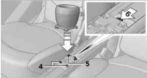
3. First insert the cupholder into the front mounts **4** and then snap it into the rear mounts **5**.
