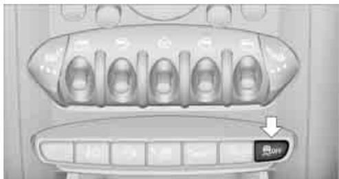
Press the button; the indicator light DSC OFF on the speedometer comes on and TRACTION is displayed on the tachometer.
