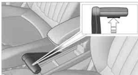
Pull upward slightly, press the button, arrow, and guide the lever down.
