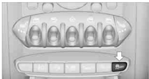
Press the button for at least 3 seconds; the indicator light DSC OFF on the speedometer comes on and DSC OFF is displayed on the tachometer. The Dynamic Traction Control DTC and Dynamic Stability Control DSC are both deactivated. There will be no more stabilizing interventions.
