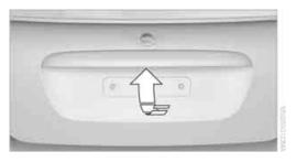
Press the button in the handle, arrow, or the button of the remote control, for an extended period. The tailgate is unlocked and can be opened.
