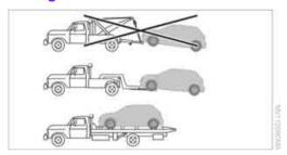
Have the MINI transported by a tow truck with a so-called lift bar or on a flat bed.
