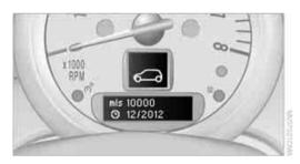
The remaining driving distance and the date of the next scheduled service are briefly displayed immediately after you start the engine or switch on the ignition.
