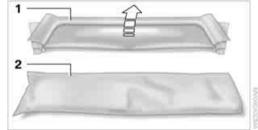
Fold the wind deflector 1 closed and slide it into the storage pouch 2.
