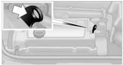
Attach the second terminal clamp of the minus/- jumper cable to the negative terminal of the battery or to the engine or body ground of the vehicle to be started.
