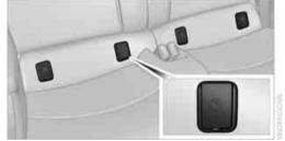
The anchor points for the lower LATCH anchors are located behind the labeled protective caps.
