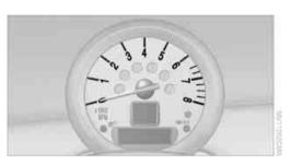
Never operate the engine with the needle in the red overspeed zone of the gauge. In this range, the fuel supply is interrupted to protect the engine.
