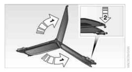
Press the locking device together until it engages, refer to arrow 2.
