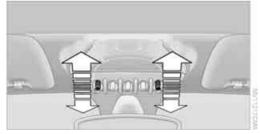
To switch the reading lamps on and off. Press the switch.
