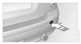
John Cooper Works with aerodynamic bumper: Pull out the bottom of the cover panel of the towing eye in the bumper, arrow.
