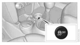
Press the button until the DSC OFF indicator lamp on the speedometer is on and DSC OFF is displayed on the tachometer. DSC is deactivated. Stabilizing and propulsion promoting actions are no longer executed.
