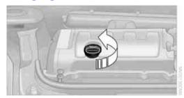
Do not add the maximum quantity of 1 US guart/1 liter of engine oil until the oil level has dropped to just above the lower mark on the dipstick, page 215.
