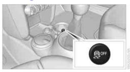
Press the button; the indicator lamp DSC OFF on the speedometer comes on and TRACTION is displayed on the tachometer.
