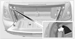
Pull on the green knob with the fuel pump symbol. The fuel filler flap is released.
