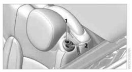
Press button 2 and fold down backrest together with the belt strap.
