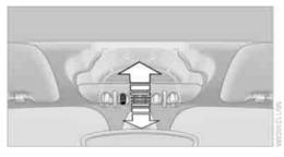
To switch the interior lamps on/off.
