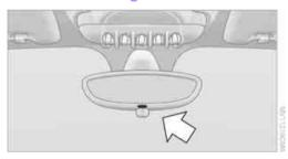
It is controlled by two photosensors:
