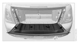
The maximum load that may be placed on the open tailgate is 175 lbs/80 kg.◀
