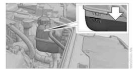
The coolant level is correct if it is between the Min and Max markings.
