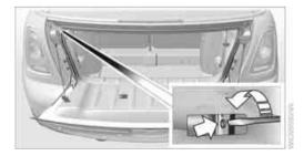
Use the screwdriver and turn the gold-colored screw, refer to arrow, one and a half turns in the direction of the arrow
