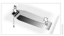
2. Insert the snap-in adapter at the front, arrow 1, and press downward, arrow 2, until
