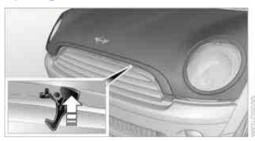
To avoid damage, make sure that the wiper arms are against the windshield before you open the hood. ◀
