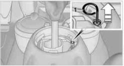
Insert extractor hook 1 from the toolkit into the loop on the passenger's side.
