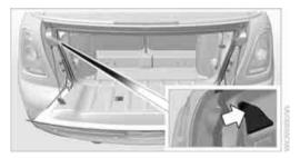
Move the convertible top to its uppermost position, refer to Loading aid page 107, and remove the cover of the luggage compartment side wall.
