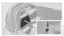
Pull on the green knob with the fuel pump symbol. The fuel filler flap is released.
