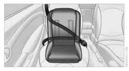
The safety belt for the passenger can be prevented from being pulled out in order to secure child restraint systems.
