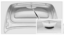
A handle recess on the interior trim panel of the tailgate make it easier to pull it down.
