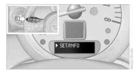
Press and hold the button until the display changes. Press the button as often as necessary until the symbol and "SET" are displayed.
