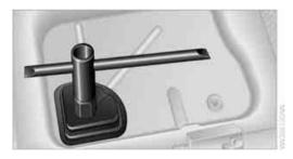
Screw the lifting handle from the toolkit onto the thread.
