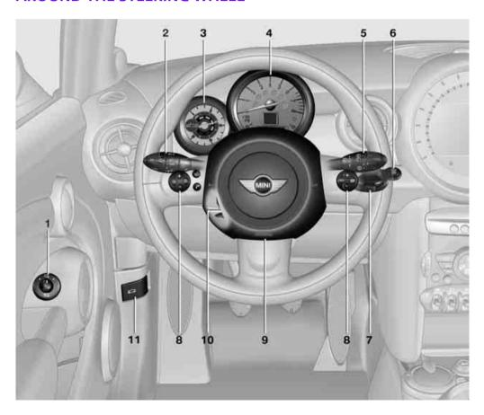
1 Adjusting the exterior mirrors, folding them in and out 48
