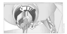
2. Push on the catch, arrow 1, and disconnect the connector, arrow 2.
