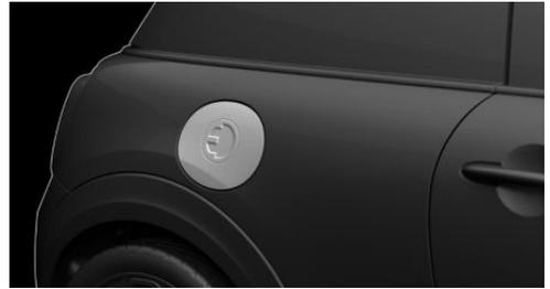
The charging socket flap is located on the right side of the vehicle.
