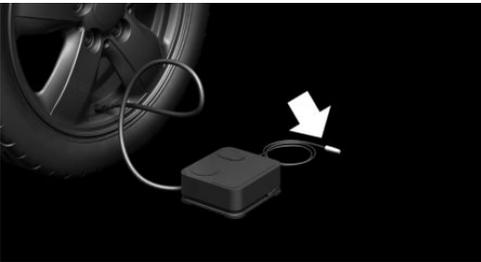
5. With standby state or drive-ready state switched on, switch on the compressor. If a tire inflation pressure of at least 2 bar cannot be reached, contact your dealer's service center or another qualified service center or repair shop. If a tire inflation pressure of at least 2 bar is reached, see Minimum tire inflation pressure is reached.
