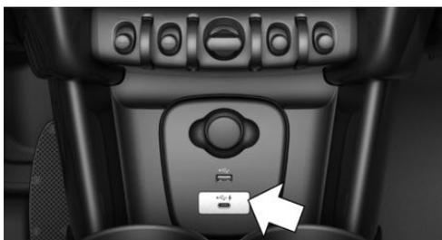
Depending on the equipment version, a USB port Type A or a USB port Type A and a USB port Type C are located in the front of the center console.
