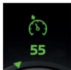
Display in the instrument cluster lights up. The current speed is adopted as the speed limit.
