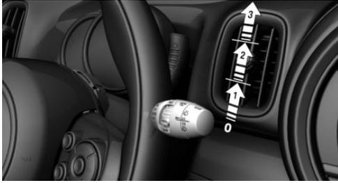
Press the lever up until the desired position is reached.
