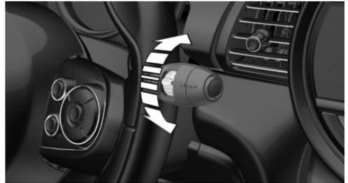
Turn the thumbwheel on the wiper lever.
