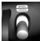
Press the MINI Driving Modes switch downward until GREEN is displayed in the instrument cluster.
