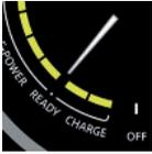
The READY display indicates that the vehicle is ready for driving. Drive-ready state in detail, refer to page 101.
