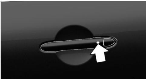
Press and hold down the button on the driver's or front passenger's outer door handle.
