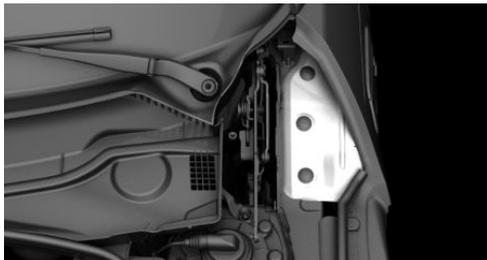
2. Loosen the nuts of the cover by hand or with the onboard vehicle tool kit, refer to page 250, and remove the cover.
