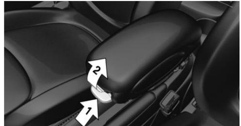
Press button, arrow 1, and swing center armrest upward or downward into the desired height, arrow 2.
