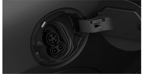
An indicator light is located on the charging socket.
