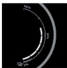
The fill level bars indicate the available charge state of the high-voltage battery when standby state and drive-ready state are switched on.
