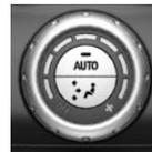
Turn wheel for air flow to the left until the control switches off.
