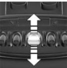
Press back the switch up to or beyond the resistance point and release it.
