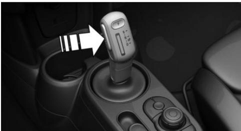
2. With the driver's safety belt fastened, briefly push the selector lever in the desired direction, past a resistance point, if needed. The selector lever automati-
