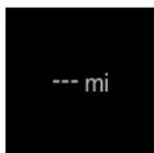
The high-voltage battery is heavily discharged. Its power output will be reduced. Heating and climate control functions will be deactivated. In this state, the exact range can no longer be calculated. A short range may still be available depending on the environmental conditions.
