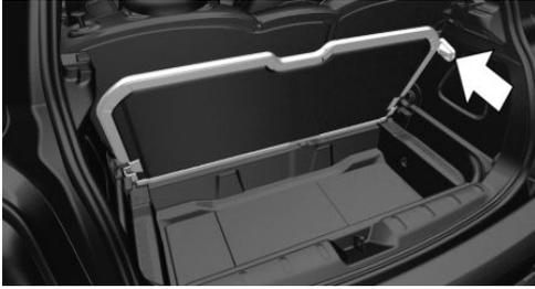
Fold up the cargo floor panel in the lower position and push it behind the locks, arrow. You've reached the maximum cargo height.
