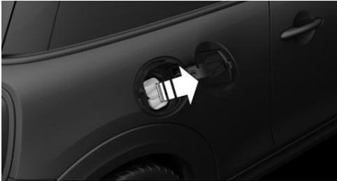
3. Remove the cover of the charging cable plug, if needed.
