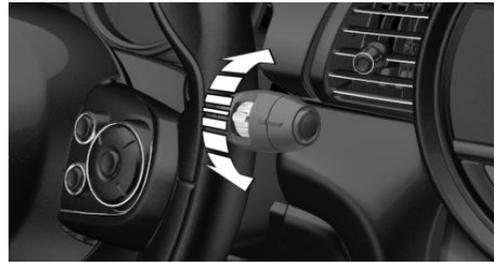
Turn the thumbwheel on the wiper lever.
