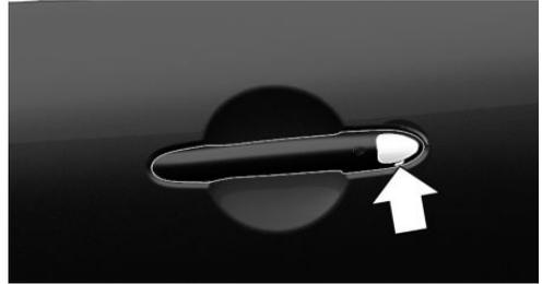
2. Unlock or lock the door lock using the integrated key.
