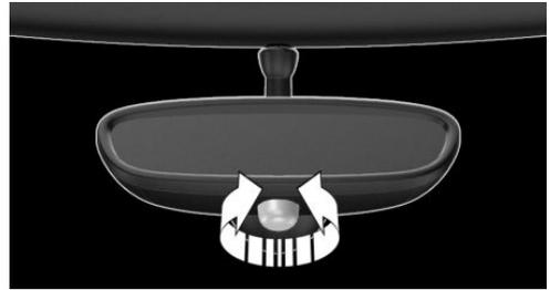
Turn the knob to reduce the blinding effect by the interior mirror.
