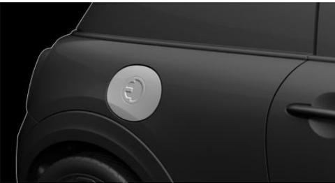
The charging socket flap is located on the right side of the vehicle.
