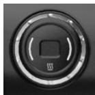
Turn the wheel to set the desired temperature.
