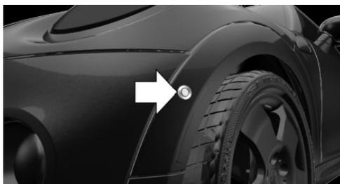
The ultrasound sensors for measuring parking spaces are located on the wheel housing.
