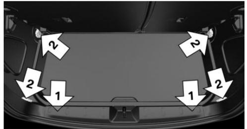
Without storage compartment package: to secure the cargo there are two lashing eyes, arrow 1, in the cargo area.
