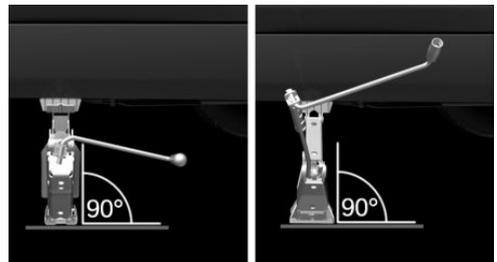
7. Crank the vehicle up, until the vehicle jack is with the entire surface on the
