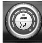
Turn the ring to set the desired air flow.
