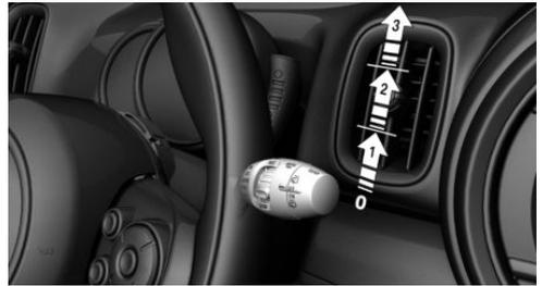
To activate: press the lever up once from its standard position, arrow 1.
