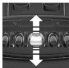
Press the switch forward beyond the resistance point and release it.
