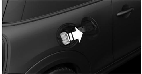
3. Remove the cover of the charging cable plug, if needed.
