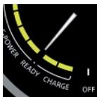
The READY display indicates that the vehicle is ready for driving.
