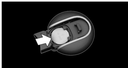
5. Insert a type CR 2032 battery with the positive side facing up.
