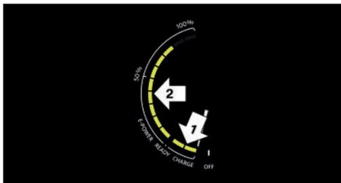
Pointer in the CHARGE range, arrow 1: display for energy recovery by coasting or when decelerating:
