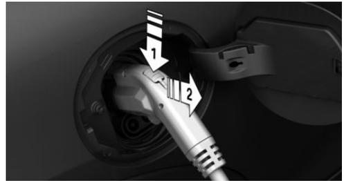
3. Remove the charging cable from the charging socket, arrow 2.
