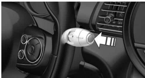
Press the button on the wiper lever.
