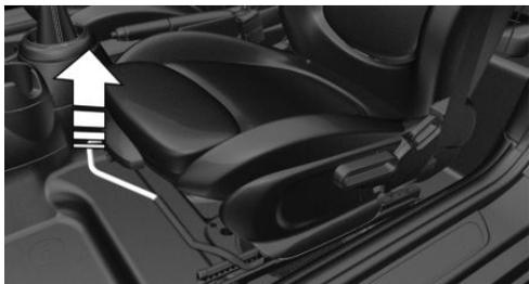
Pull the lever and slide the seat in the desired direction.
