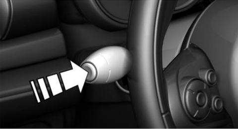
Press the button on the turn signal lever. Information is displayed in the instrument cluster.
