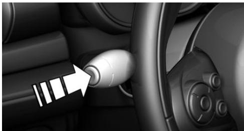
Press the button on the turn signal lever.
