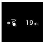
The expected range for the energy stored in the high-voltage battery is continuously displayed in the instrument cluster.
