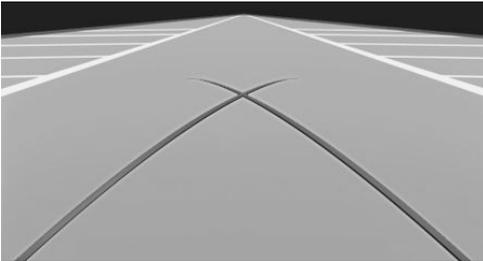
Turning radius lines can be superimposed on the image of the rearview camera.
