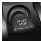
Pressing the Start/Stop button switches standby state on or off.
