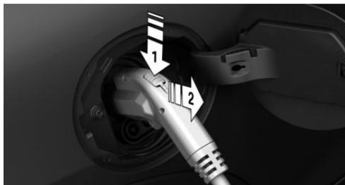
3. Remove the charging cable from the charging socket, arrow 2.
