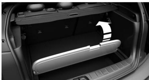
2. Grasp the cargo floor panel in the rear and fold slightly upward.
