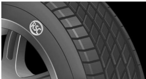
RSC label on the tire sidewall.
