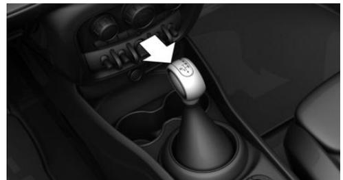
Press unlock button on the front of the selector lever, arrow.
