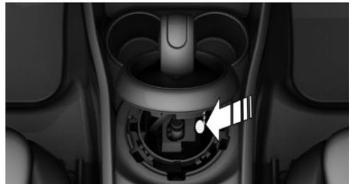
4. Move the selector lever slightly toward the rear; to do this press the unlock button on the front of the selector lever. Release the release lever.
