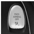
▷ The indicator lamp lights up when a child is properly seated in a child restraint fixing system or when the seat is empty. The airbags on the front passenger side are not activated.
