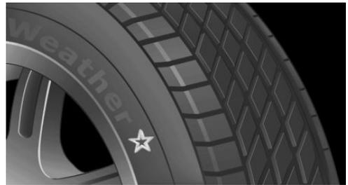
For each tire size, the manufacturer of the vehicle recommends certain tire brands. These can be identified by a star on the tire sidewall.
