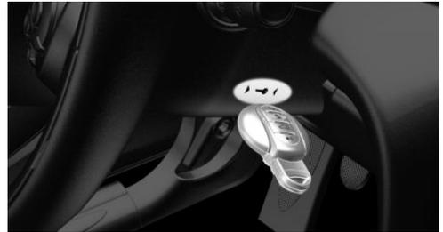
Steptronic transmission: if a corresponding Check Control message appears, hold the remote control, as shown, against the marked area on the steering column and press the Start/Stop button within 10 seconds while pressing the brake.
