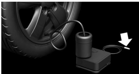
6. With operating readiness switched on or the engine running, switch on the compressor.
