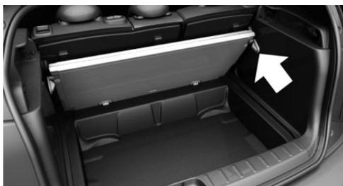
Fold up the cargo floor panel and press behind the locks on the left and right, arrow. You've reached the maximum cargo height.
