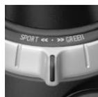
Turn Driving Dynamics Control to the right until GREEN Mode is displayed in the instrument cluster.
