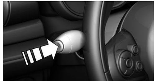
Press and hold button on turn signal lever.
