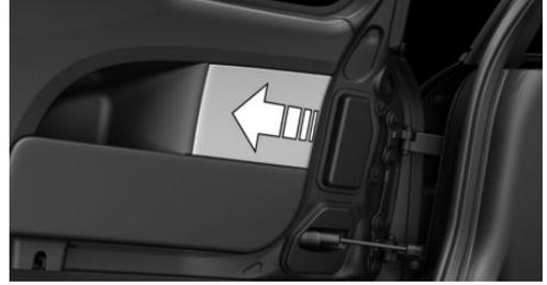
3. Press the latches together in the direction of the arrow, arrow 1, and remove the bulb holder.
