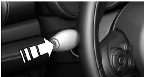
Press and hold button on blinker lever.
