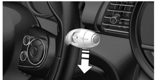
The lever automatically returns to its initial position when released.
