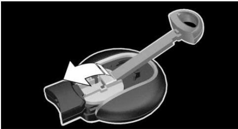
4. Insert a battery of the same type with the positive side facing up.
