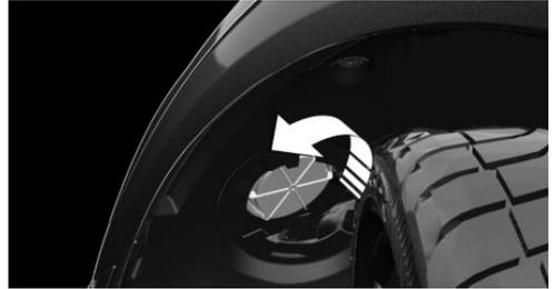
4. Pull bulb holder out of the bulb housing; if needed, loosen it with small tilting movements if possible.
