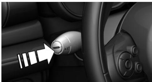
1. Depending on the equipment, turn the light switch into position
