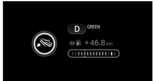
Instructions tell you to switch to a more fuel-efficient driving style when you back off the accelerator.
